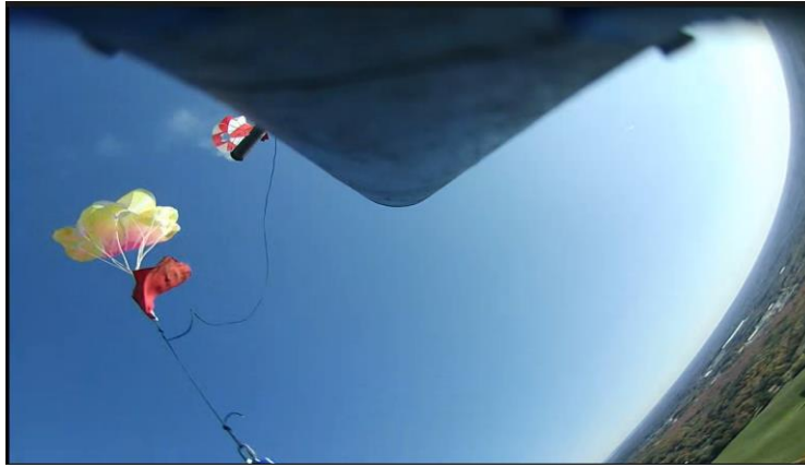
Image 3.4.4.4: Second frame confirming smoke venting from Main Parachute Bay at T+14.40s
