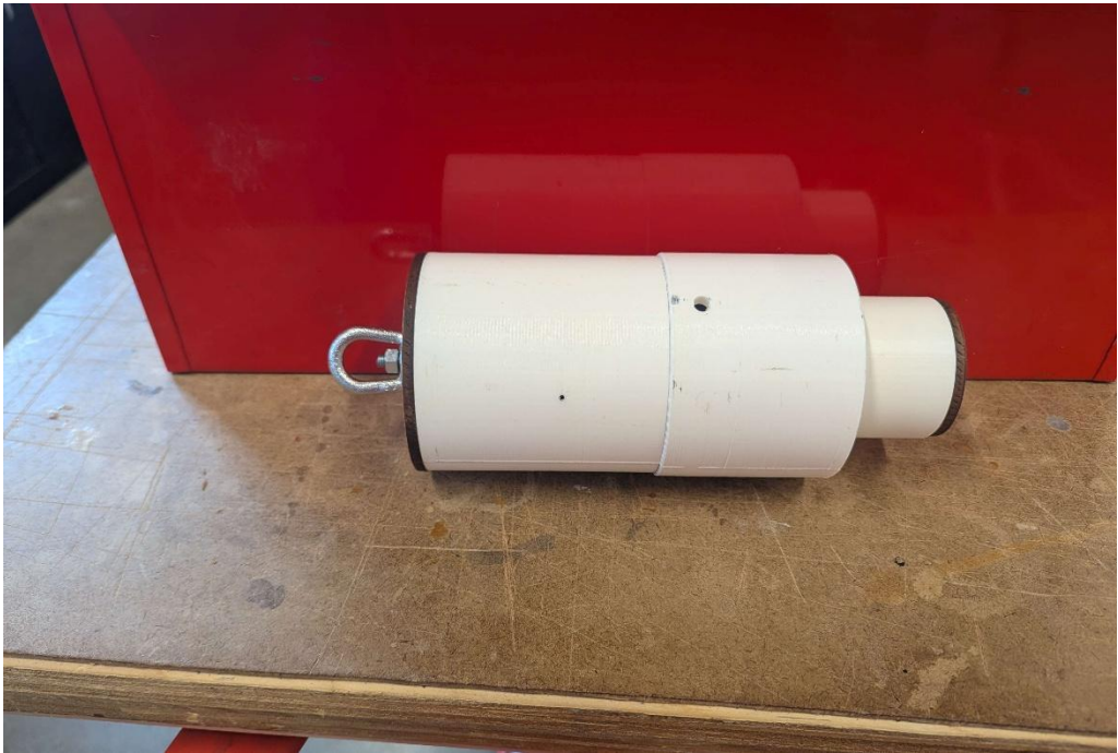
Image 4.2.1: PERR-C during partial assembly, including fitment testing of ballast payload assembly prior to VDF
