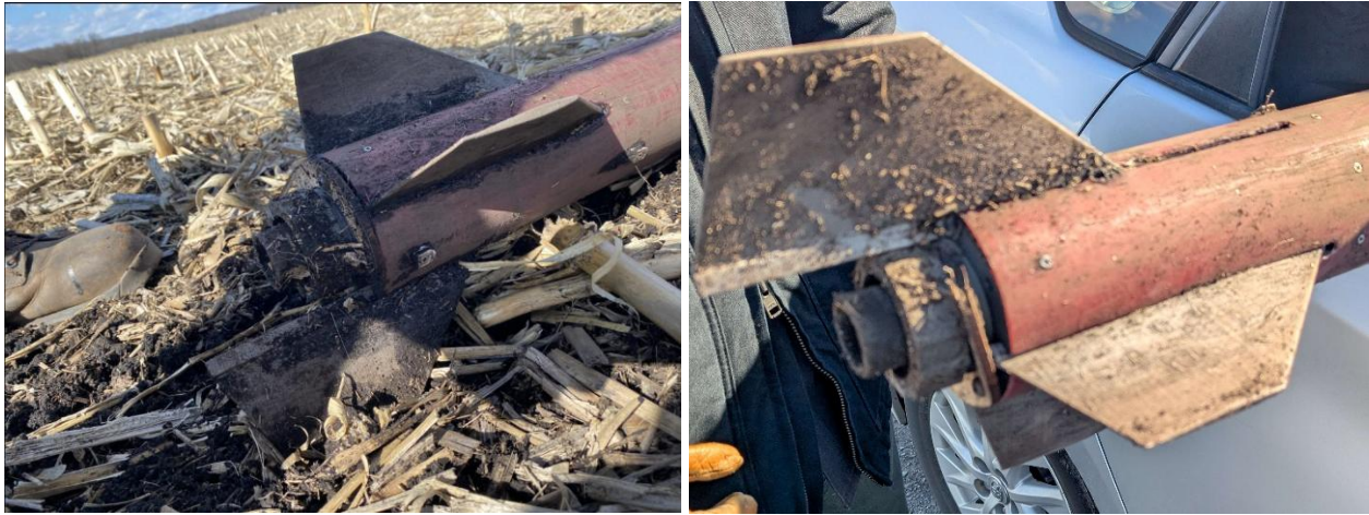
Image 5.5.1: Image of Fin pushed through Fin Retainer on landing (left) and after returning to the flight line (right)
