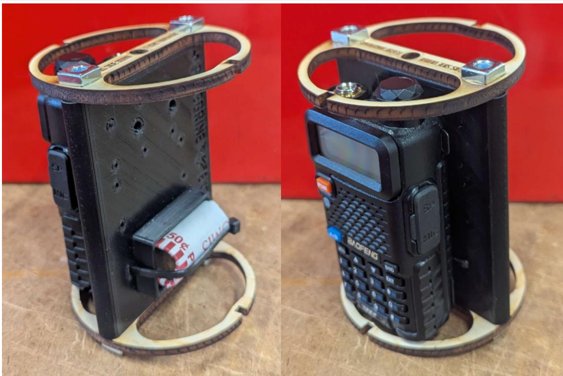
Image 4.2.2: PEP test package assembled prior to flight. Pennies were used to simulate payload mass and test the structural integrity of the battery mounting system. Square nuts are used with engraved reliefs in the bulkheads to align and assemble the package evenly.
