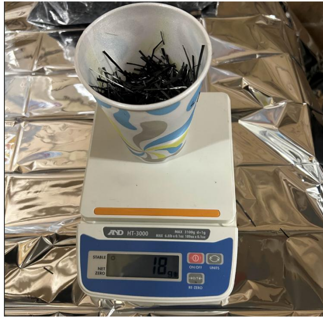
Image 4.2.5: Weighing out Carbon Fiber Tow
