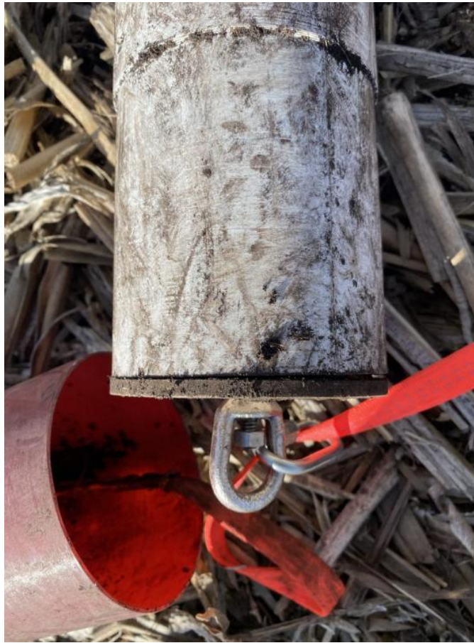
Image 5.5.14: PERR-C Locknut near end of threaded rod after landing
