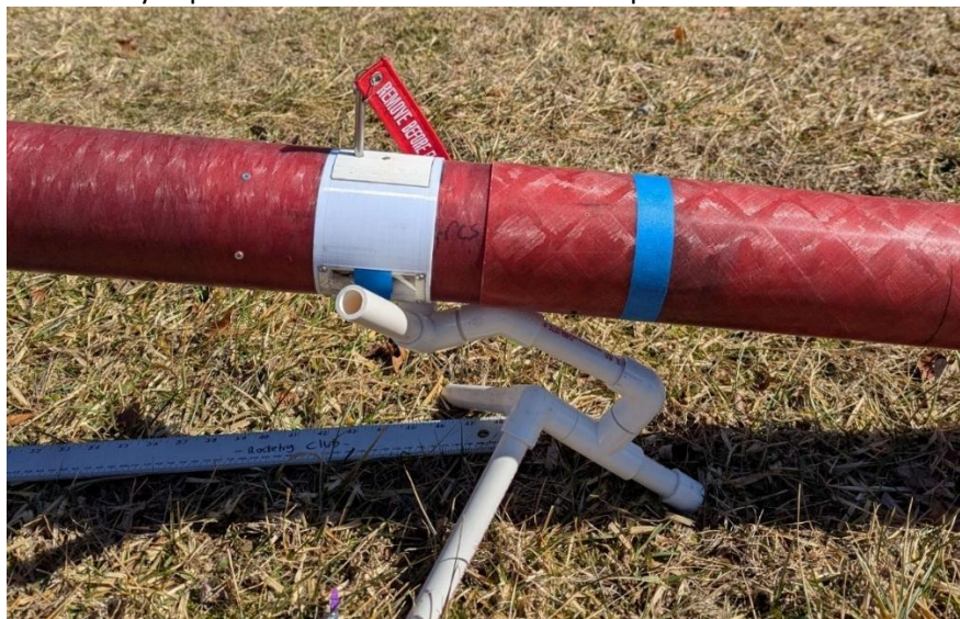
Image 7.1.3: Result of Partial Success Drogue Ejection
