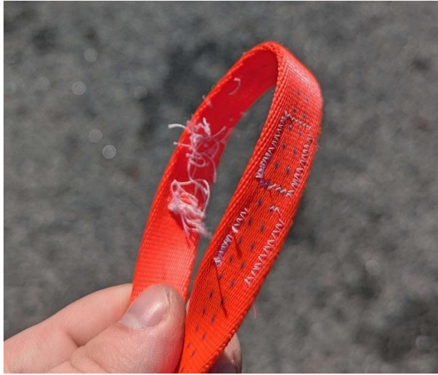
Image 5.5.10: Damage to Main Parachute Tether and mechanism of failure diagram
