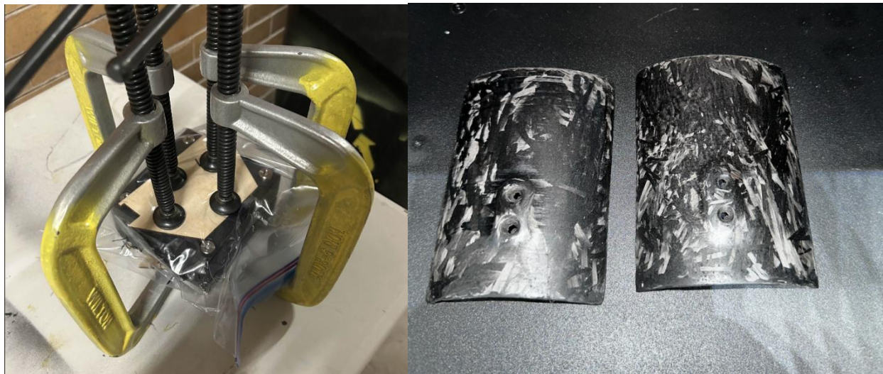
Image 4.2.6: Clamped mould and Final results of ACS Flap
