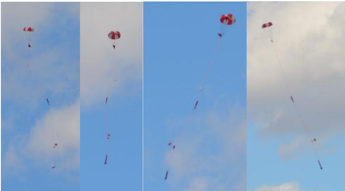
Image 5.5.11: Sequence showing PERR-C sliding down the main tether after tether failure.
