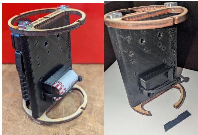
Image 5.5.12: Photos of PERR-C Sled Before (left) and After (right) Flight
