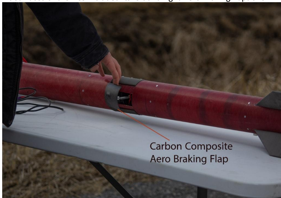
Image 4.2.3: Image of Full vehicle assembled with the flap manually actuated
