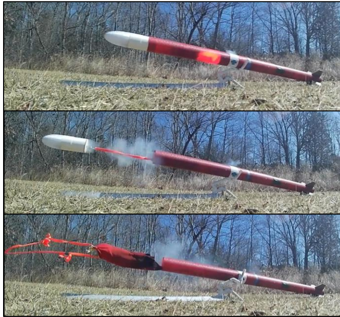
Image 7.1.2: Sequence of Main Parachute Ejection during Pop Testing
