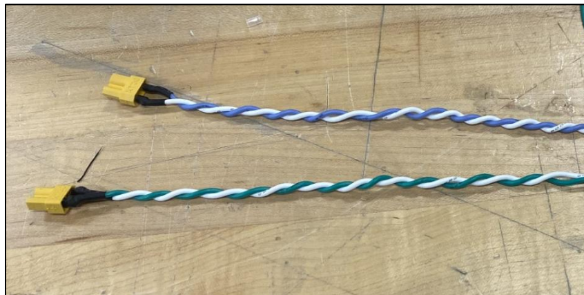
Figure 3.2.1.1A: Example of Twisted Wire Pairs and XT-30 Connectors.
