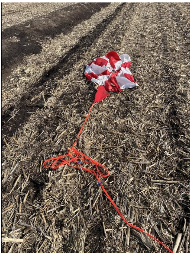
Image 5.2.7: Main parachute and tether tangled in the vegetation
